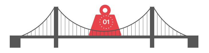
Place a small weight on the deck of your suspension bridge model. Remember that you model is not made from steel cables like real suspension bridges so don't overload it. Once the weight is placed on the deck, go through each component and note down whether you think it is in tension or compression.
