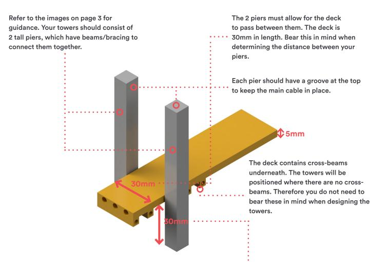
The maximum size allowed for each tower is  $60 \times 15 \times 105$  mm (w x l x h). You will require 2 identical towers for the model.
