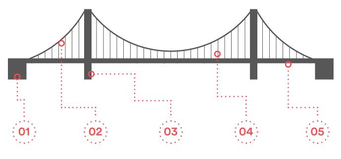
Anchorages Anchorages are the connection point for the cables, keeping them tight. They must have a large mass and are usually constructed from concrete or rock. Main Cables The main cables are made up of hundreds of wires bundled together! They stretch from one anchorage to the other and are the components that the deck 'hangs' from.
